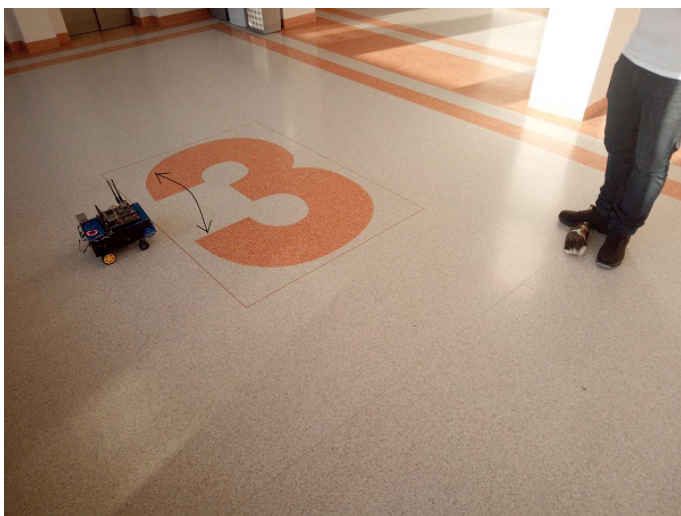
Figure 10. The robot does not detect the pet and starts turning around.
