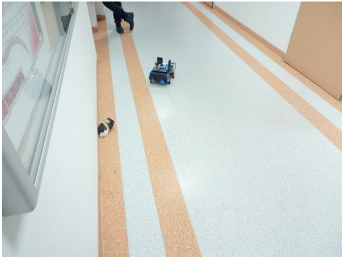
Figure 8. The robot detects the pet and moves towards it.
