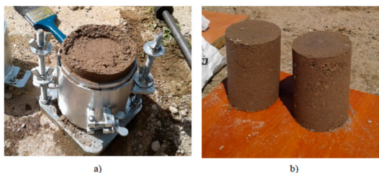
Figure 6. Preparation of the samples made of fine aggregate with cement: cylindrical form (a); samples (b).
