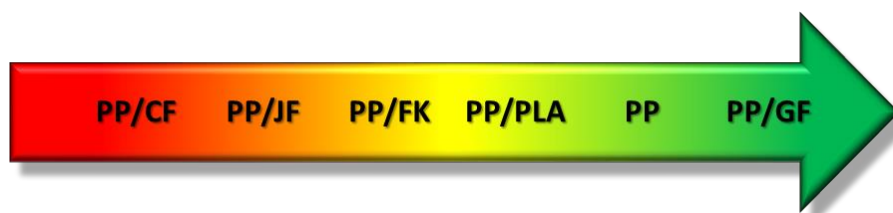
Figure 5. Schematic diagram of recommended material variants for EUR-pallet in terms of water footprint.
