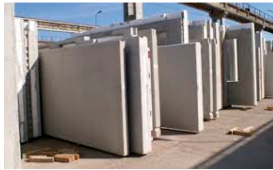
Figure 2. Prefabricated elements storage.
