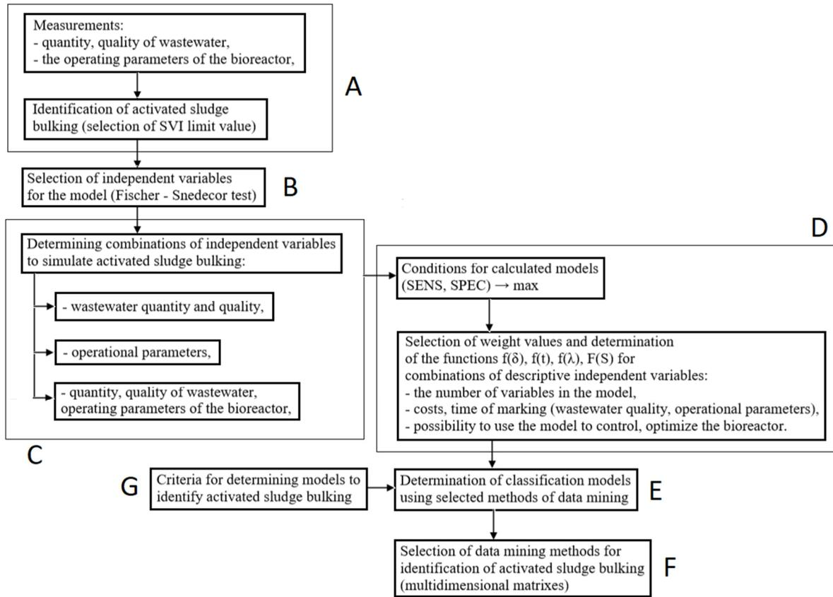
**Figure 1.** A schematic of the soft sensor system for selecting a data mining method for simulating sludge bulking.
