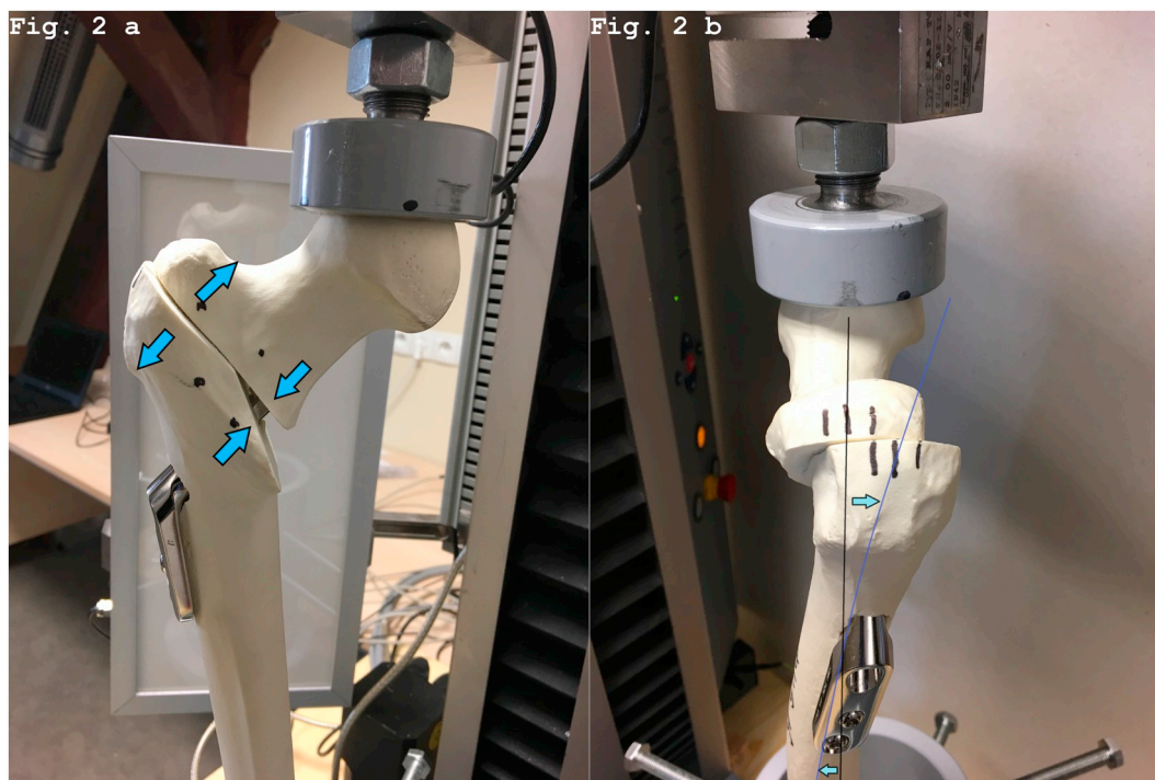
Fig. 2. Rotational failure of the DHS.
