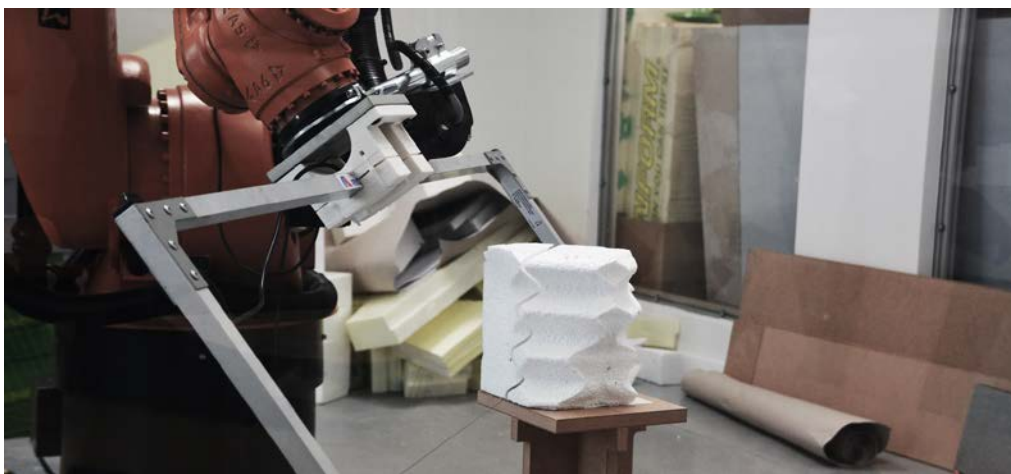
Figure 6: The process of hotwire-cutting with robotic arm.
