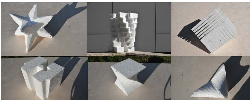
Figure 7: Forms achieved with wire-cutting.
