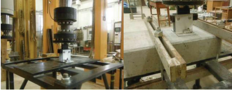
Fig. 4. Laboratory test stands for steel and concrete bases
