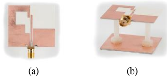
Fig. 7. Photographs of the fabricated antenna prototype: (a) front view, (b) 3D view.
