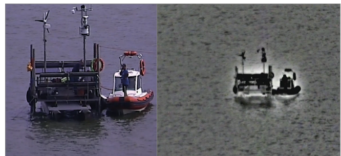
Fig. 12. Image from long-range cameras during the day: visible light camera (left), thermal imaging camera (right)
