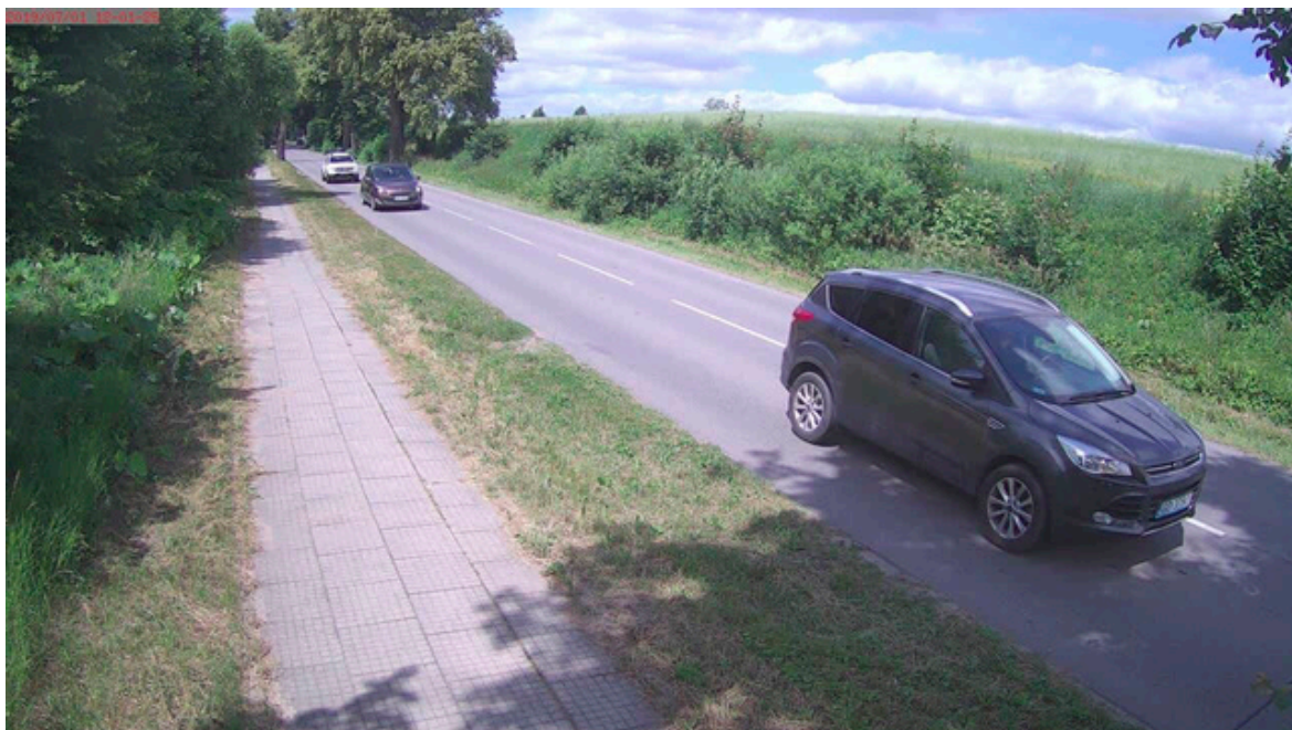
Figure 16. The test road section—a view from the camera mounted in the test system. The first measurement tubes are mounted at the trees visible in the back, the second pair is positioned near the bottom right corner of the photo.
