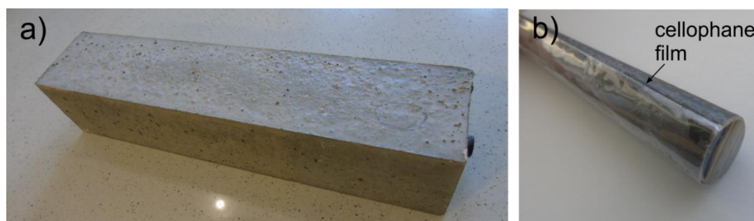
Figure 7. Experimental investigations: (a) Exemplary beam model, (b) rod covered with cellophane film before casting into concrete.
