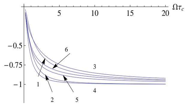
Figure 3. Variations in the background dimensionless temperature  $\frac{T_4\gamma_\infty u_\infty^2}{EQ_0(\gamma_\infty-1)^2(Q_\rho+(\gamma_\infty-1)Q_T)}$  as a function of  $\Omega\tau_c$ , after an impulse has gone away.  $E = \int_{-\infty}^{\infty} v_1^2 dt$  measures the energy of an impulse per unit mass of a medium.
