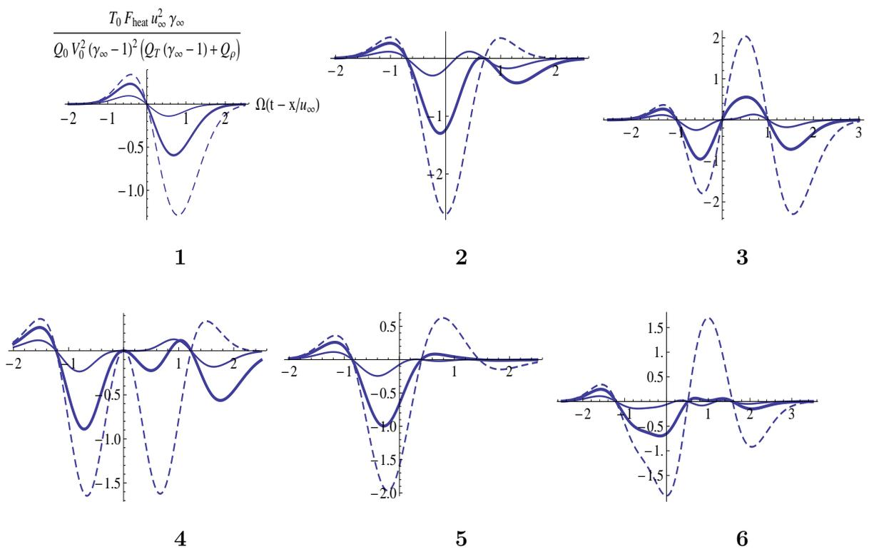
Figure 2. The dimensionless acoustic force of heating (cooling) caused by impulses Eq.(16)(1)- Eq.(21)(6). The normal lines correspond to  $\Omega\tau_c = 0.2$ , the bold lines correspond to  $\Omega\tau_c = 1$ , and the dashed lines correspond to  $\Omega\tau_c = 100$ .
