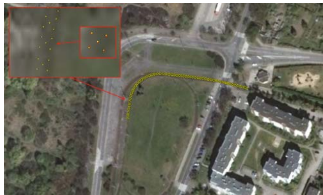
Figure 6. Aligned recording results for a selected section of the tramway track loop in Gdansk – source: prepared by the authors
