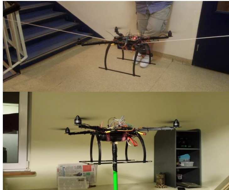
Fig. 10. Testing Stabilization with quad-copter
