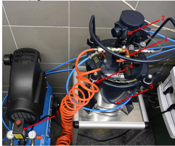
Fig. 2. System of the abrasive suspended matter's preparation: 1- compressor, 2- power transmission of the mixer's rotor, 3- pressure regulating device regulator inside the tank, 4- the tank's cover, 4- suspended matter's tank, 5- bowl of the tank.
