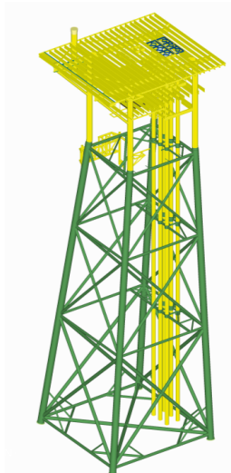
Fig. 12. Geometric model of production platform – isometric view
