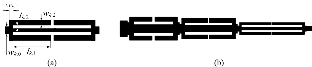
Fig. 5. CMRC-based three-section impedance matching transformer used for verification purposes: (a) compact microstrip resonant cell (CMRC) cell, (b) transformer geometry.
