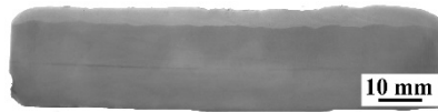
Figure 7. An example view of a cross-section of the layer made by an Omnia electrode in the air, with etching using Nital 4%.
