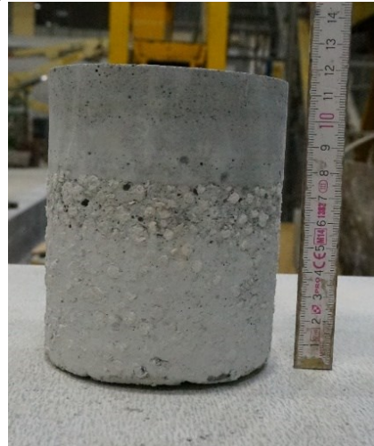
Fig. 6. Changes in thickness of self-leveling screed and EPSC layer: a) measurement of detached screed layer 10.37 \div 28.59 mm, b) EPS concrete layer (140 mm) in a core sample, 10 mm of screed, c), EPS concrete layer (75 mm) in a core sample, 42 mm of screed.
