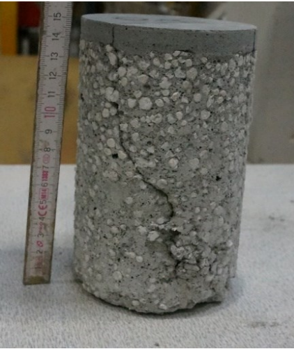
Fig. 6. Changes in thickness of self-leveling screed and EPSC layer: a) measurement of detached screed layer 10.37 \div 28.59 mm, b) EPS concrete layer (140 mm) in a core sample, 10 mm of screed, c), EPS concrete layer (75 mm) in a core sample, 42 mm of screed.
