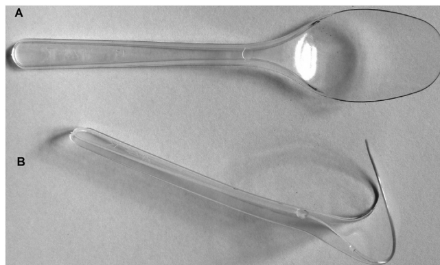
Fig. 1. Appearance of a disposable transparent teaspoon made of polystyrene (A) before and (B) after being used to mix a hot beverage.
