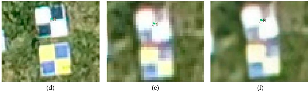
**Figure 4.** Images of ground-control points from the Mavic Pro: a) GCP-5 at 55m, b) GCP-5 at 110m, and c) GCP-5 at SR and from the Phantom 4 Pro: d) GCP-5 at 55m, e) GCP-5 at 110m, and f) GCP-5 at SR.
