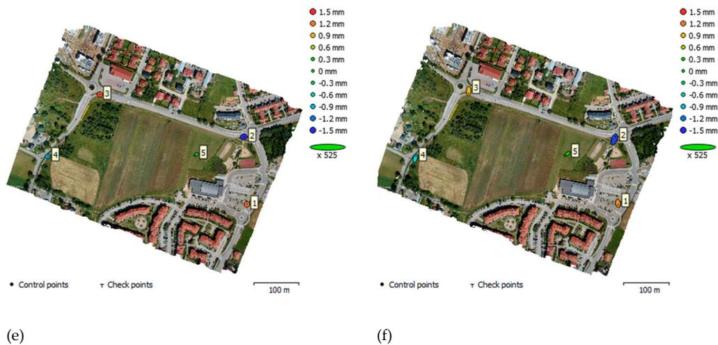
**Figure 5.** GCP locations and error estimates for the Mavic Pro: a) at 55m, b) at 110m, and c) SR and for the Phantom 4 Pro: d) at 55m, e) at 110m, and f) SR. Z error is represented by the ellipse color. X,Y errors are represented by the ellipse shape.
