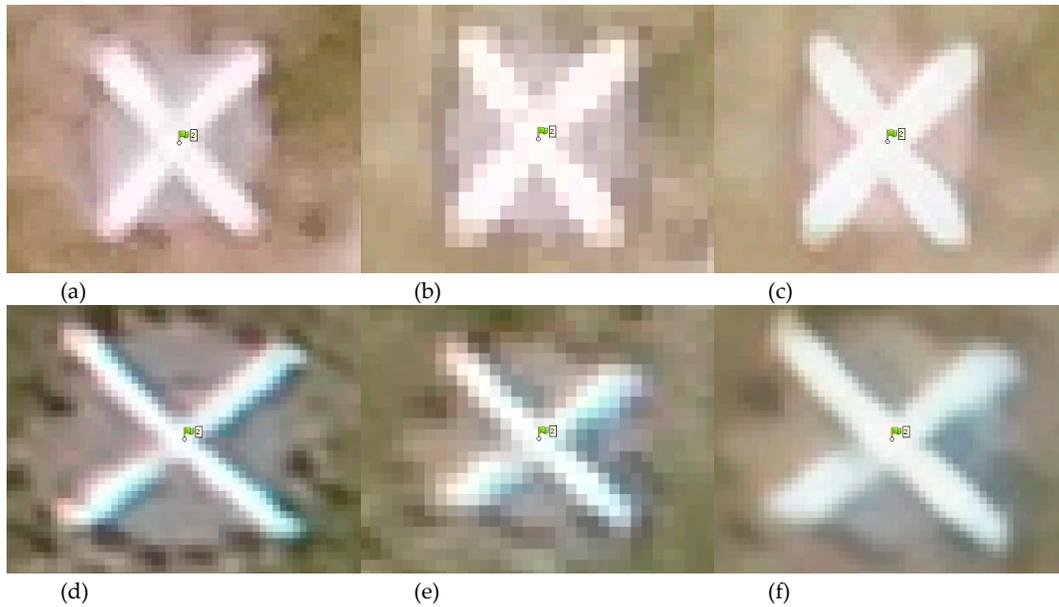
**Figure 3.** Images of ground-control points from the Mavic Pro: a) GCP-2 at 55m, b) GCP-2 at 110m, and c) GCP-2 at SR and from the Phantom 4 Pro: d) GCP-2 at 55m, e) GCP-2 at 110m, and f) GCP-2 at SR. SR: super resolution.
