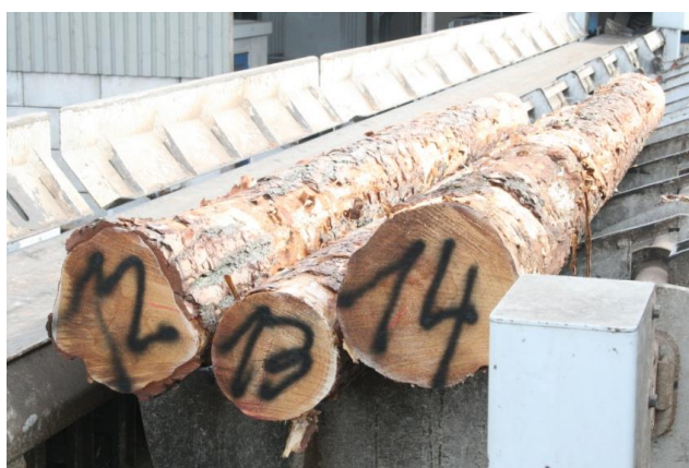
Fig. 1 Marked Scotch pine logs ready for sorting operation.
