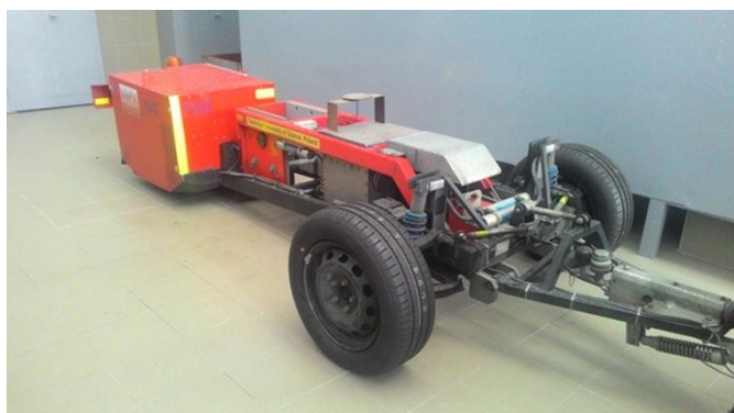
Fig. 2. R2 Mk.2 trailer for measuring the rolling resistance coefficient of tires and pavement [11]
