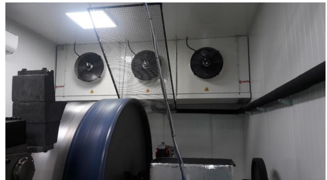
Fig.7. Thermostatic chamber used in the tire testing laboratory of the Gdańsk University of Technology (own material)
