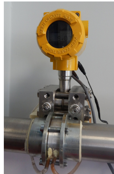
Fig. 10. APR-2000/ALW transducer mounted on the laboratory stand.
