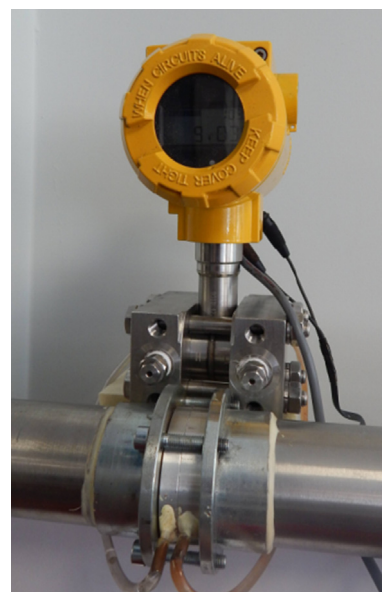
Fig. 10. APR-2000/ALW transducer mounted on the laboratory stand.
