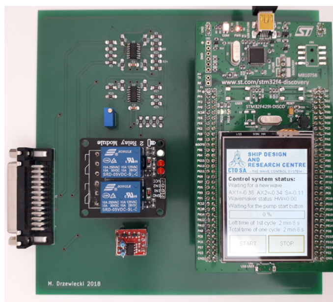
Figure 11. The wave maker embedded system, equipped with a Graphical User Interface [7].
