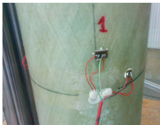
Figure 2. View of a pair of strain gauges at point 1—strain gauges in the picture covered with adhesive to protect against mechanical damage and moisture.
