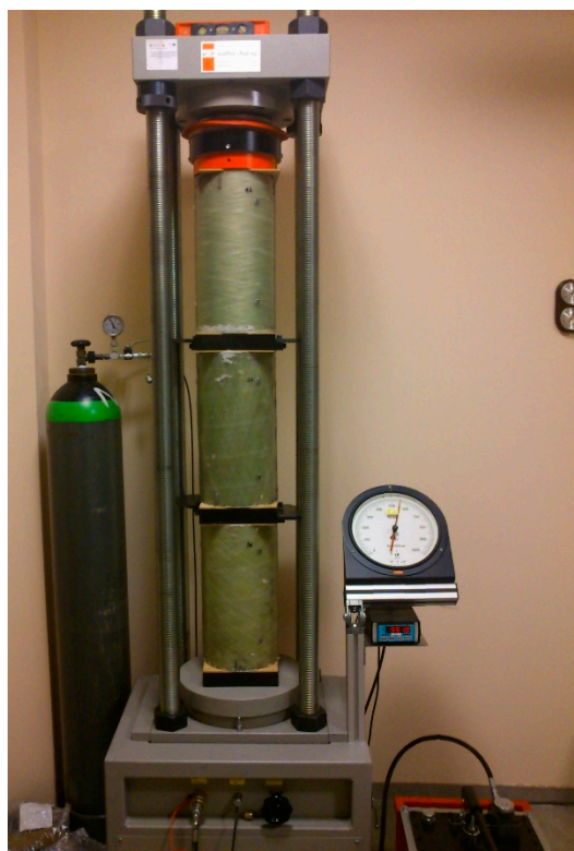
Figure 17. Testing of rheological deformations (creep and shrinkage).
