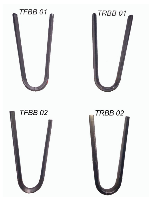
Figure 5. Specimens after bending tests.
