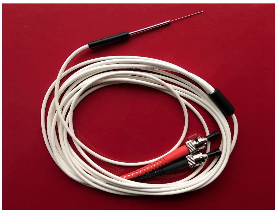
Figure 1. Laser Doppler intramuscular fiber-optic perfusion probe.
