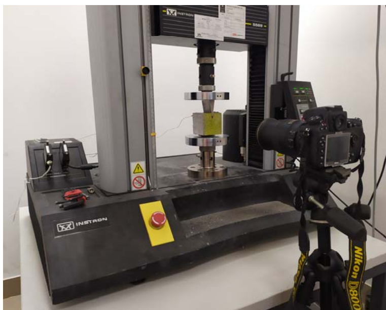
176 177 178 Figure 3: View on the DIC testing station. Digital NIKON D800 camera is mounted on a tripod 179 perpendicularly to the concrete cubic sample during Wedge Splitting Test (WST) carried out 180 using Instron 5569 static machine 181
