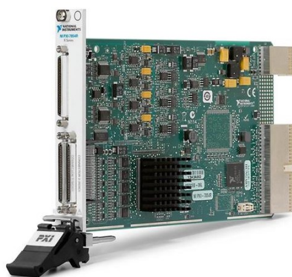
Figure 1. Field-Programmable Gate Array (FPGA) PXI-7854R illustration [11].
