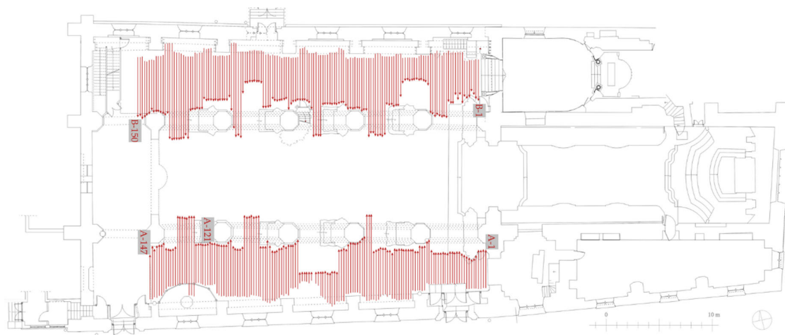
Figure 6. Plane view of the church with ground penetrating radar (GPR) traces in the south (traces A-1 to A-147) and north (traces B-1 to B-150) aisles.
