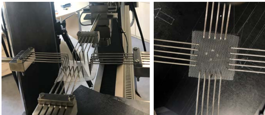
Fig. 1. Set up in biaxial tests
