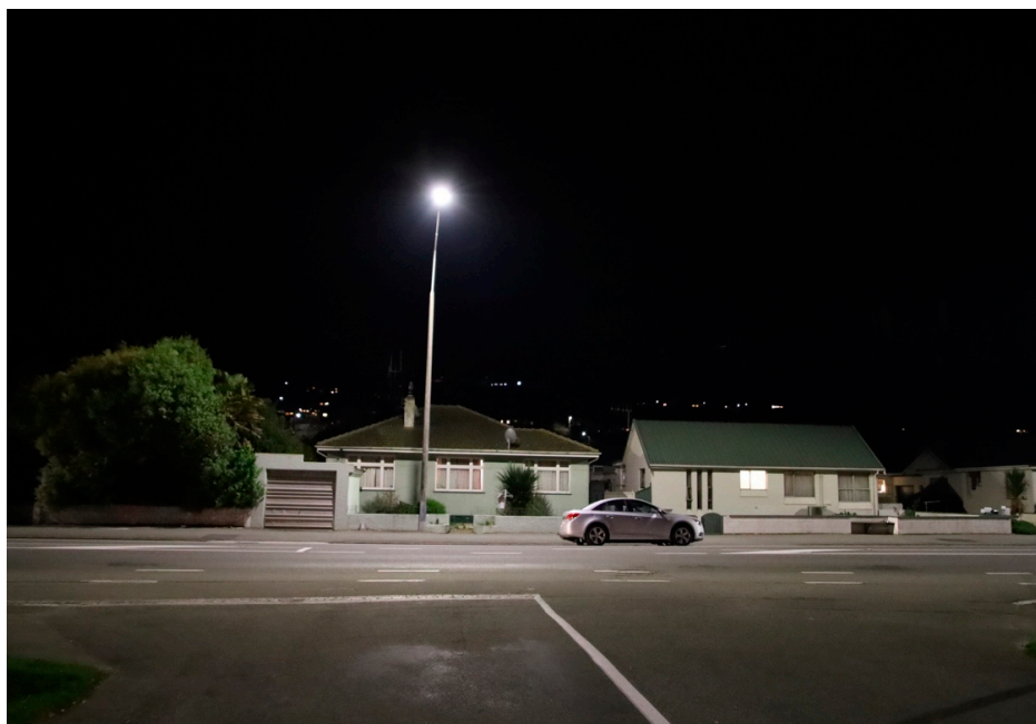
Figure 5. Light trespass/light spill from unshielded 4000 K LED street lighting entering the windows of residential properties in Oamaru/NZ. Source: Damien McNamara.
