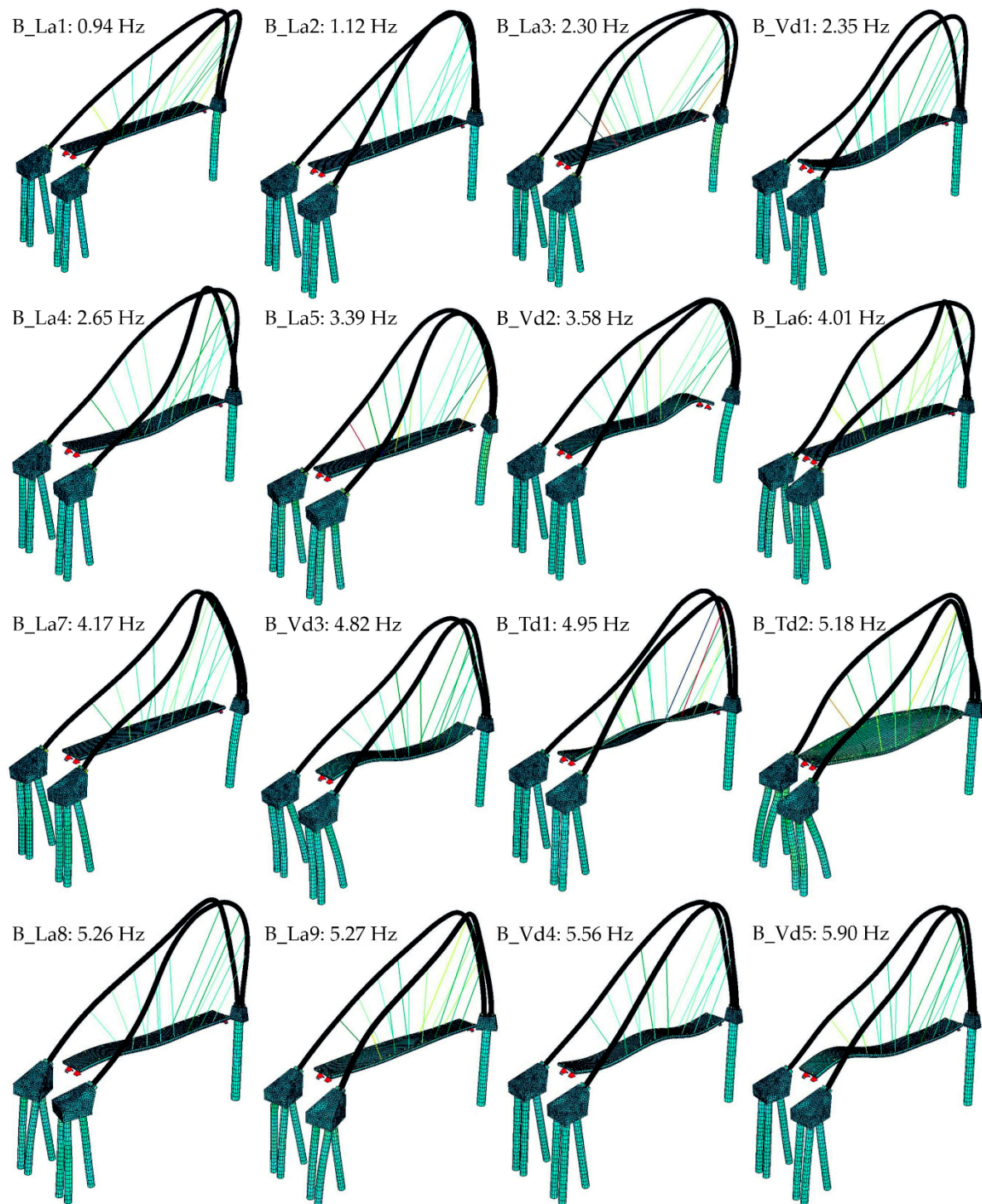
Figure 14. FEM eigenvectors and eigenvalues of the footbridge above the University Route in Bydgoszcz.
