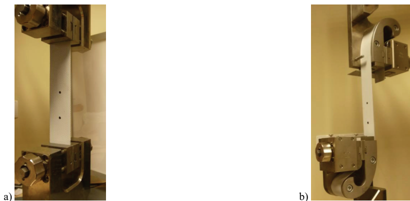
Fig. 2. Types of grips used in uniaxial tensile tests: a) flat, b) curved
