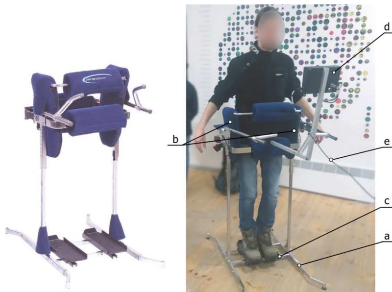
Fig. 1. Unmodified parapodium (left), and JStep during testing (right): a) mechanical structure, b) sensorized pillows, c) sensorized feet platforms, d) visualization panel, e) USB cable to PC.
