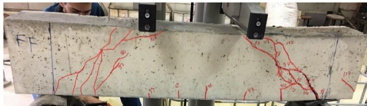
Fig.12: Beam (B4) at failure
