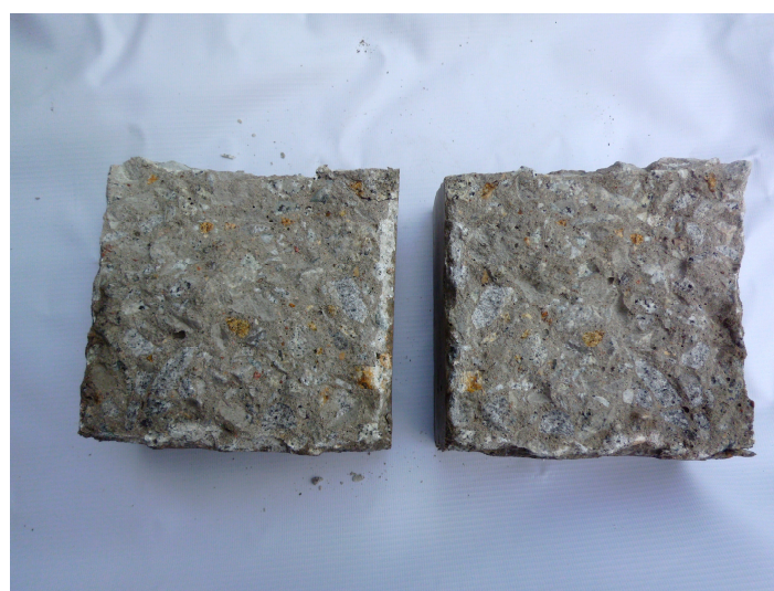
Figure 12. Fracture sample treated the lubricating oil.
