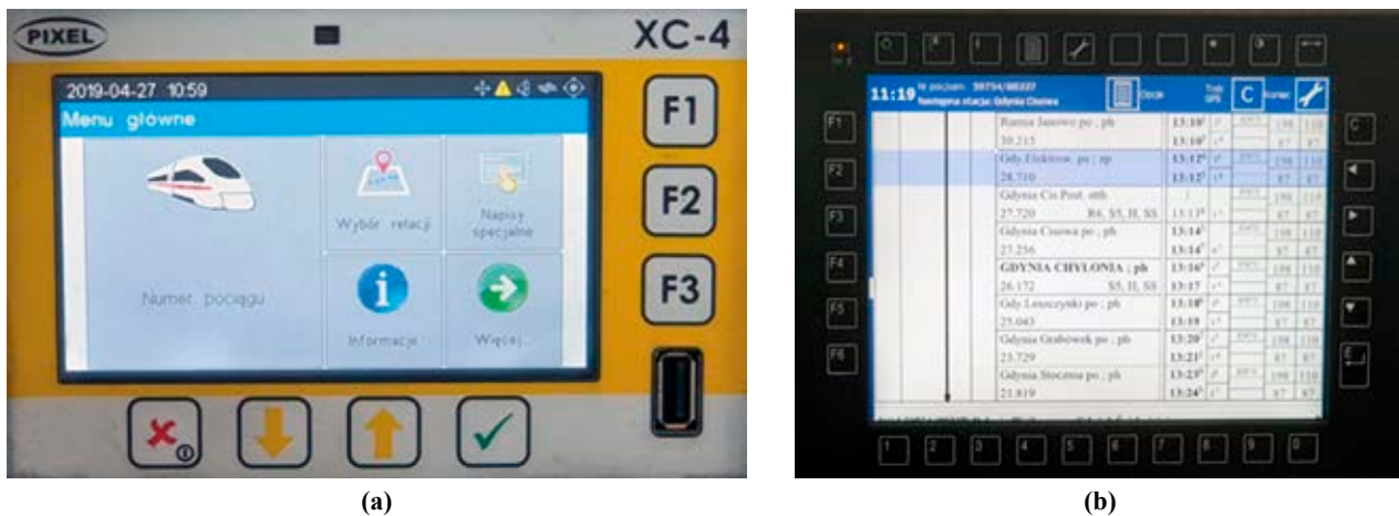
Figure 3. The PIXEL on-board computer in the EN71-035 train (a) and the timetable display for the driver, made by the R&G, in the EN71-045 train (b)
