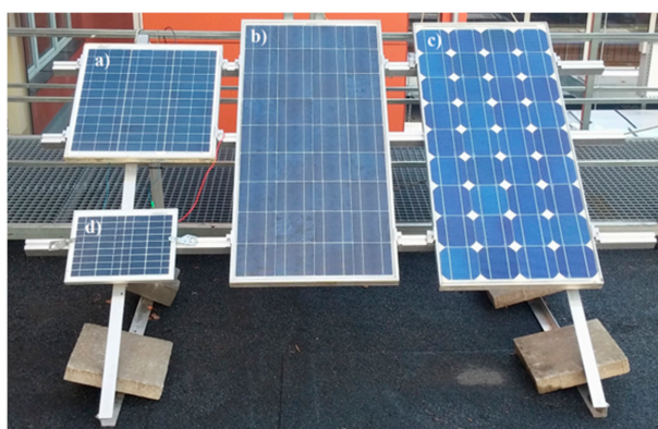
Figure 1. Photovoltaic modules chosen for the annual field study: (a) MWG-30, (b) AP-7105, (c) STP-085, (d) CLC010-12P.
