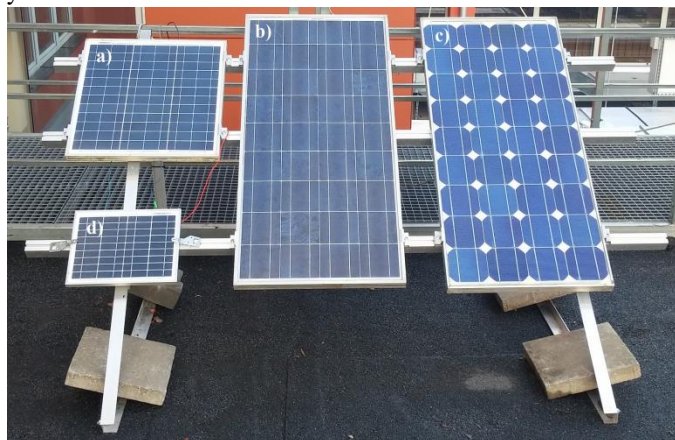
Fig. 3. PV modules used for field studies: a) MWG-30, b) AP-7105, c) STP-085, d) CLC010-12P
