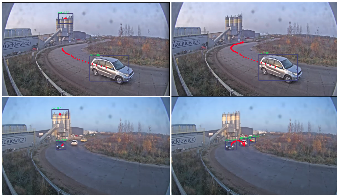
Figure 9. Qualitative results: original model (column on the left) and the fine-tuned model (column on the right). Fine-tuned model allows for the detection of the vehicles in the far end (2nd row), which also results in a longer tracking period of the vehicles (1st row). Also, note that the false-positive detection on the factory building (left column), is removed after adaptations stage.
