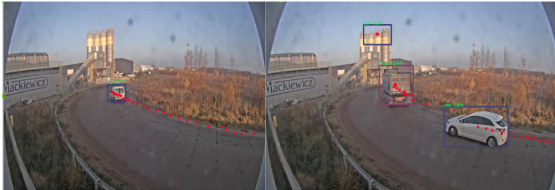
Figure 3. Even though some vehicles are being tracked for many frames, they are detected by an object detector with low confidence (car on the left image with confidence = 0.55, truck on the right image with confidence = 0.44). Note that false positive detection (car detected in the upper part of the right image) can be removed using the background model.
