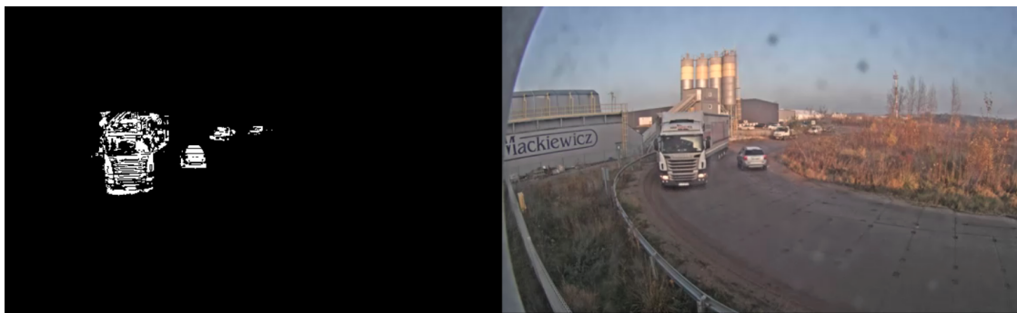
Figure 4. Background/foreground separation using background subtraction algorithm [42].
