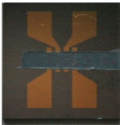
Figure 6. Gas sensing layer comprising \text{TiO}_2 nanoparticles and graphene flakes: photo of the sensor made by painting on a silicon substrate with four-point gold contacts.
