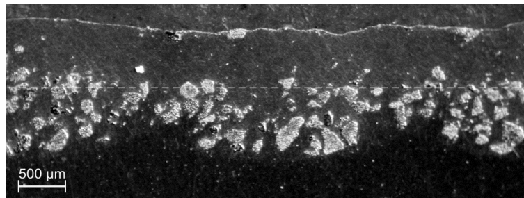
Figure 7. Cross-section through a composite layer based on Al6061 alloy with TiC powder; experimental conditions: I = 400 \text{ W/mm}^2 , v_{sc} = 10 \text{ mm/s} , m_p = 6 \text{ g/min} .
