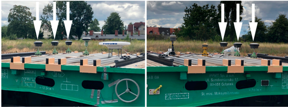
Figure 3. Global Navigation Satellite System (GNSS) receivers by Leica mounted on the mobile surveying platform.
