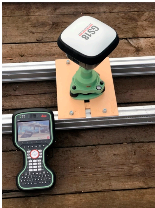
Figure 2. A LEICA GS-18 receiver used during the surveys.
