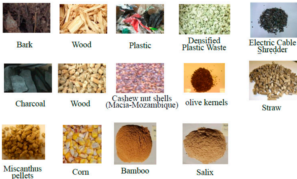
Figure 3. Types of materials used for HiTAG/HiTSG conversions.
