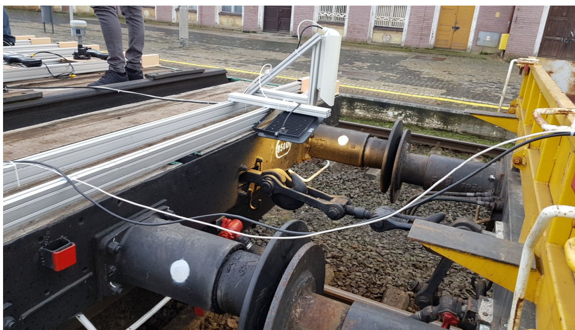
Figure 19. The coupling connecting the power car with the platform car.
