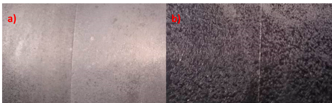
Figure 5. Effects of the substrate on the quality of the produced phosphate coating: (a) 235JR steel without chromium and molybdenum; (b) 42CrMoS4 + QT chromium-molybdenum steel.
