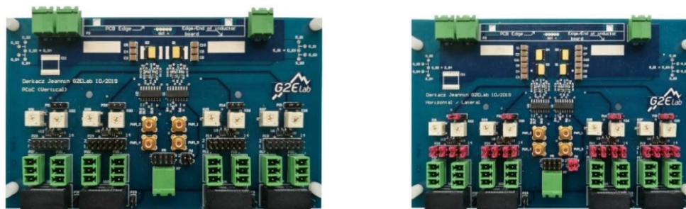
Fig. 12: 2 prototypes realized: one PCoC-GaN and one 2D realization
